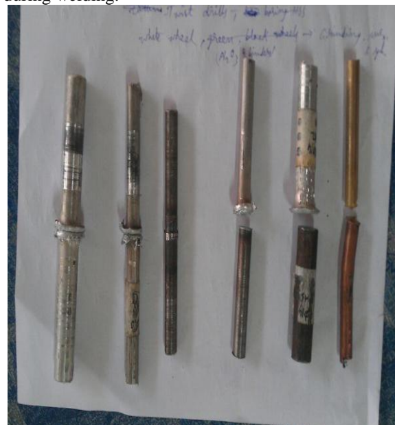
Specimens welded at 1250 rpm
