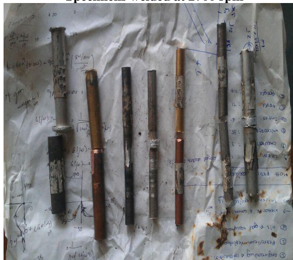
Specimens welded at 2700 rpm
